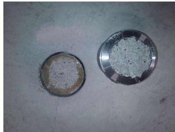
(b) Epoxy failure (X).
