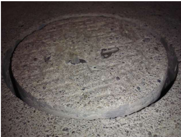
(c) Roughening of core surface.
