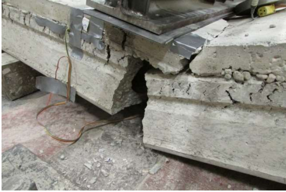
(a) FMA2-1 (strand rupture).
