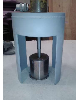
(b) Disk attachment to pull-off apparatus.
