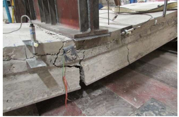
(b) FMB2-2 (strand rupture).
