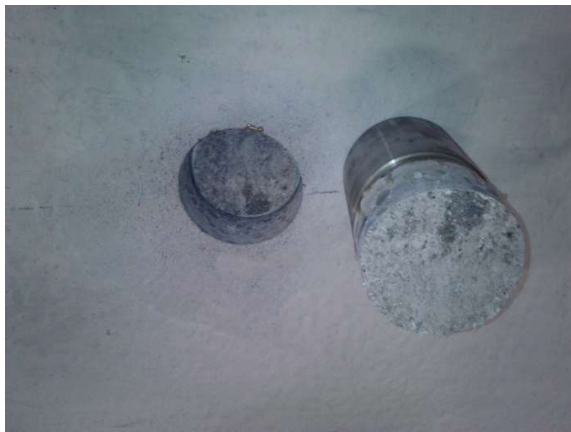
(a) Interface failure (I).
